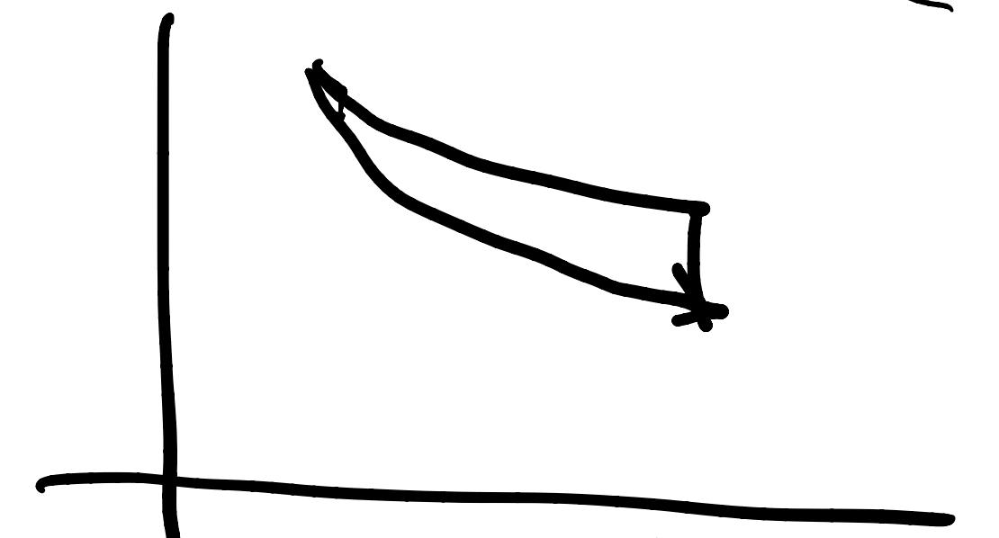
$$-nR \ln\left(\frac{V_f}{V_i}\right) = C_V \ln\left(\frac{T_f}{T_i}\right)$$
